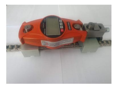
Tool for checking and effectively indicating the tension to be applied on the chain transmission. Necessary to physically calculate the type of tension in Kg and N.
